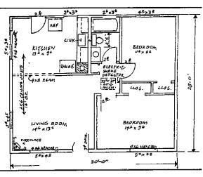
For an addition or renovation, show schematic floor plan of entire house to scale. Dimensions and details are needed only where new work is to be done Wall Key for Remodels:
